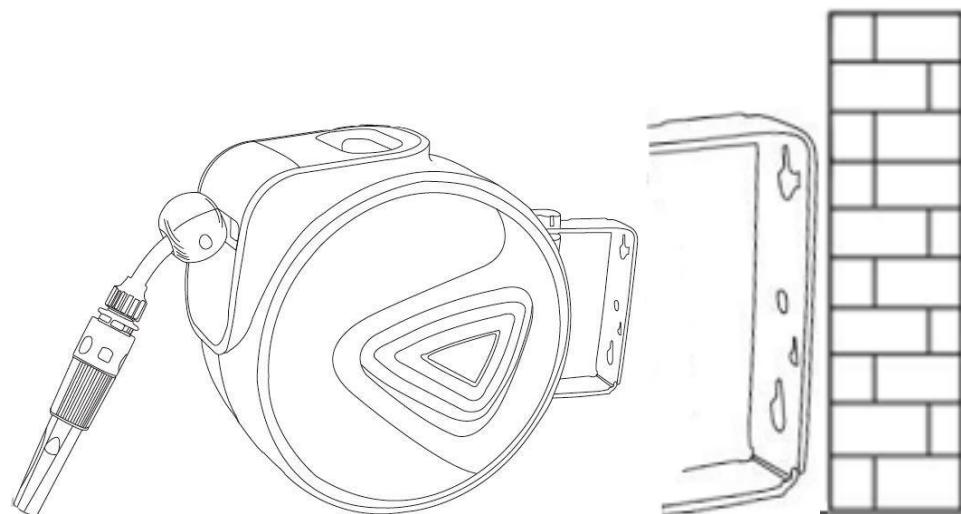
Drill 2 x 8 mm holes to match the holes located in the Mounting Bracket.
