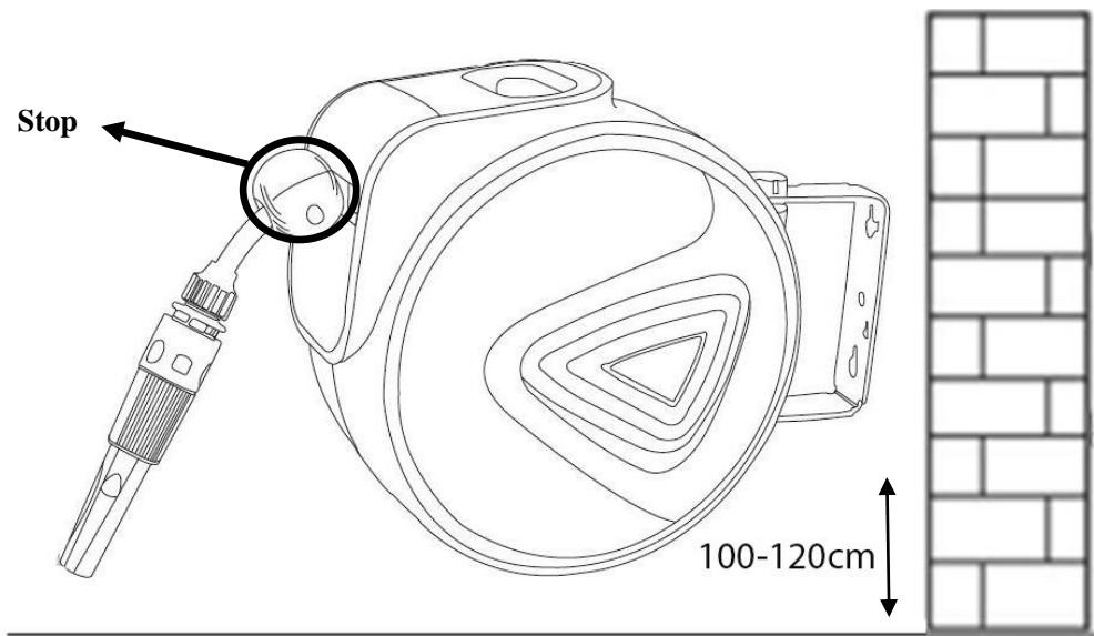
It is recommended to install the mounting bracket 100-120cm from the mounting bracket to floor.
